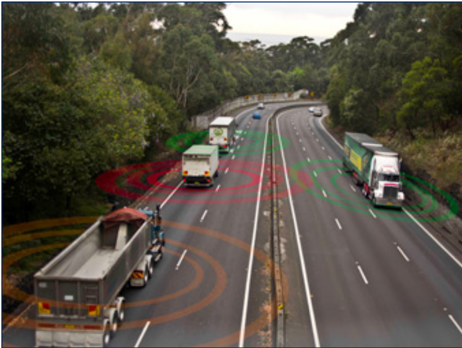
Figure 3. The Cooperative Intelligent Transport Systems (CITS) project in the Illawarra allows communication between vehicles and infrastructure. (Source: John Wall)
